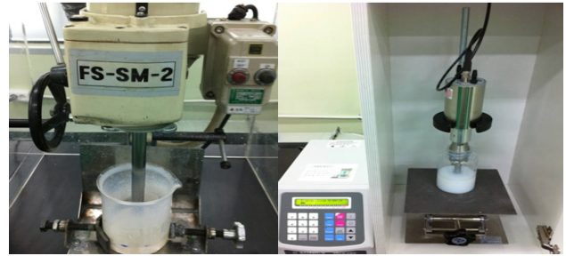
Fig. 4. Compounding process of organic-inorganic sols.
